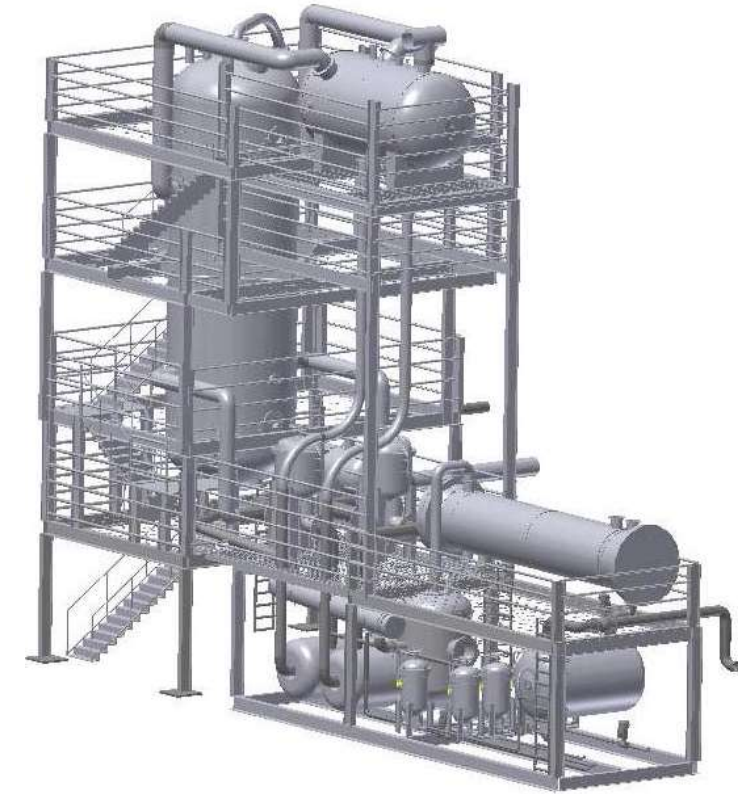
FT REACTOR MODULE
